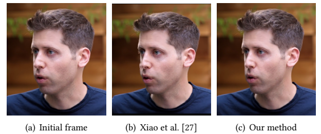
Figure 6: Comparison with the baseline method. Given a frame from a portrait video (a), Xiao et al. [27]'s reshaping method produces artifacts (b) near the tip of the nose because the nose occludes the side face, while our method can still generate satisfactory results (c) with the same reshaping parameter.
